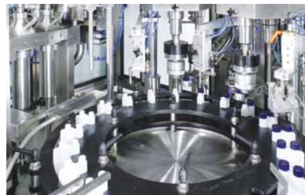
Servo-driven piston dosing and sub-level filling nozzles, 2 closing stations, N 2 gasification and final inspection
