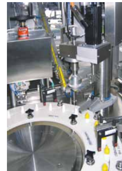
Ceramic rotary piston driven by 2 separate servo motors
