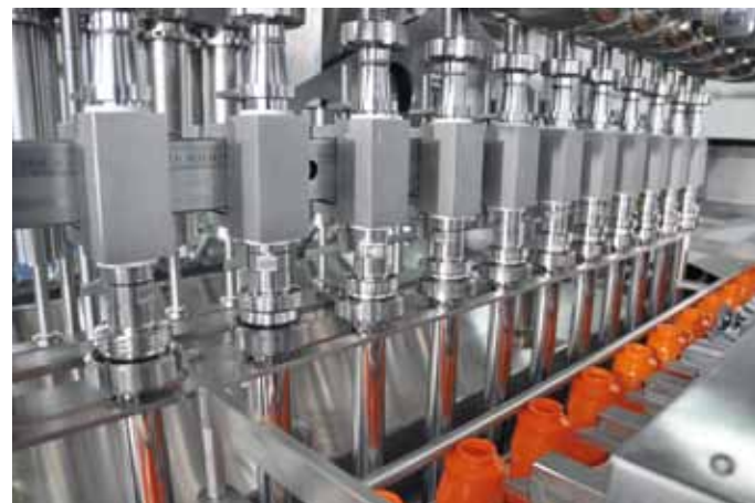
Auto-CIP* Automatic retraction of filling nozzles in CIP position
